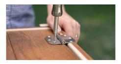
Screw hinges into the body of the cooler.
