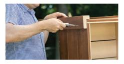
Line up L-shaped decking pieces so the edges are flush with the top of the cooler body. Using a Phillips head screwdriver or drill attachment, carefully connect the L-shaped legs to the cooler body using 1.5" screws.
